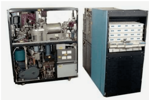
Late 1960s IBM 1360 ("Cypress") Photo-Digital Store processor. Used by the CIA among other organizations for mass storage. CHM X1385.97L
